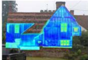
Fourteen thermographic images have been stitched together and overlaid on the photo.
